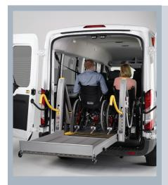
Worldwide unique design due to the specially manufactured aluminium profile lifting arms.
